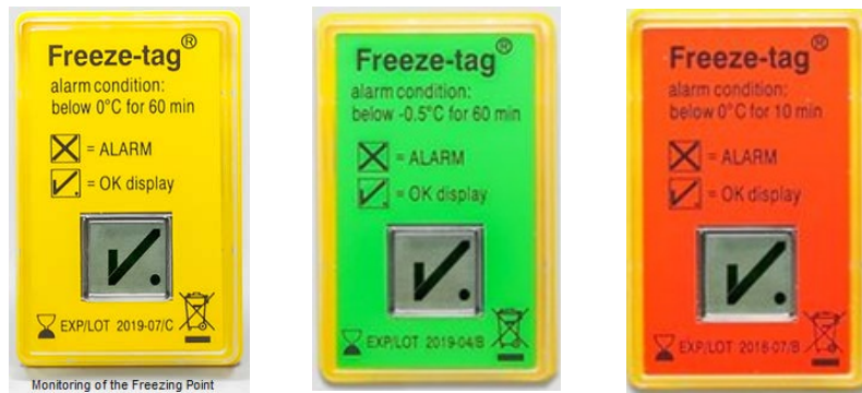
Figure 29. Freeze-Watch Indicators (Freeze-tag)
