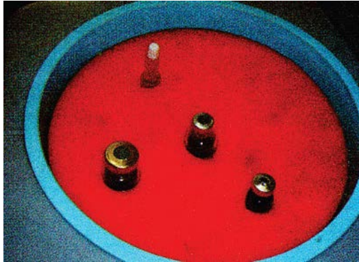
Figure 36. Foam Pad with Vials in Top of Vaccine Carrier
